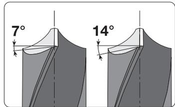
The optimal clearance angle for the job depends on the material – a harder material requires a drill with a smaller clearance angle while a softer material can have a larger angle. The size of the drill is also a determinant for the selection of the optimal clearance angle. A larger drill should have a smaller clearance angle while a smaller should have a larger one.
