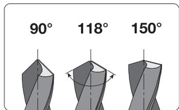
A drill bit needs to have the right lip clearance angle to cut the material. The clearance angle varies from 7° to 14°. A drill with a larger clearance angle cuts more easily, but if the angle is too large, vibrations will occur and the drill will cut irregularly and quickly become dull. If the clearance angle is too small, the drill will not cut at all, but will become hot and rapidly destroyed.
