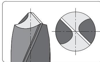
All the components are made with high precision which ensures that the lengths of the two cutting edges will be equal within close tolerances. This is an essential requirement so that the two edges will work in the same way and so that the drill will bore a round, straight hole, which is not larger than the drill diameter.
