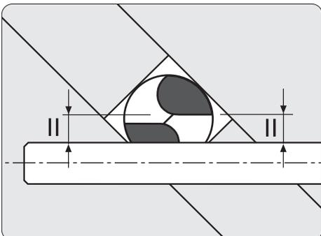
The cutting edges should be parallel to the pin in the Magnifier.
