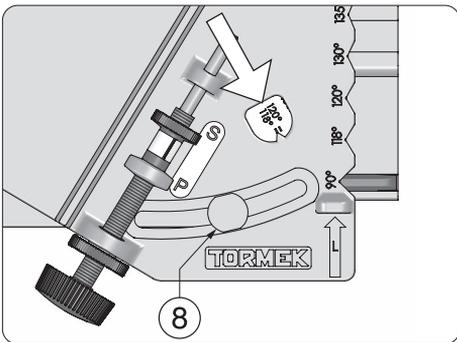
Set the guide on the selected point angle and lock with the wheel (8).
