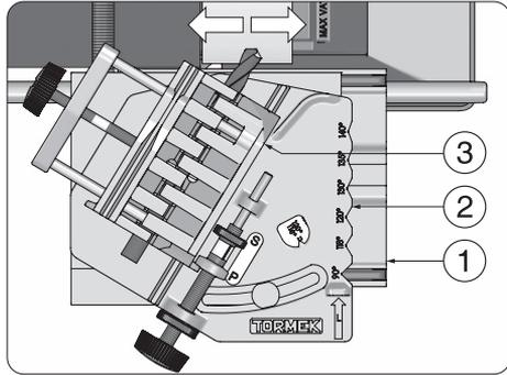
The drill is mounted in a Drill Holder (3) on a Guide (2), which in turn runs on a Base (1). You move the drill across the grindstone – the grinding automatically takes place on the highest spot of the stone.
