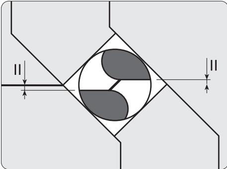
The high precision drill holder consists of two identical parts. The drill will be exactly centered and both of the cutting edges will be sharpened exactly to the same shape.
