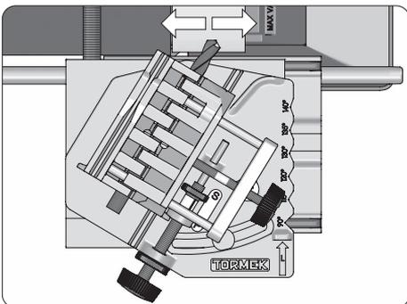
After grinding one facet, the drill holder is turned 180° and the other facet is ground to an identical shape. Now both of the two primary facets are ground.
