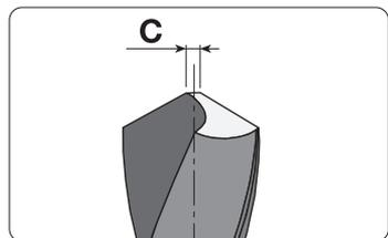
More expensive drill bits are ground with special points of various types. These drills must be re-sharpened in their original production machines or in special machines, which are available only at a few specialist sharpening shops. They can also be re-shaped to a 4-facet point with the Tormek attachment.
