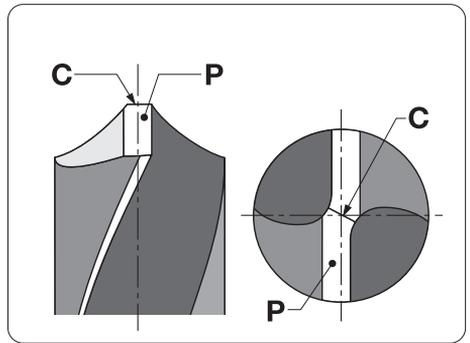
You can tell by the decreasing sound when the primary facets **P** are ground equally. How far they are ground over the centre does not matter. It is important that they are ground symmetrically. The primary facets should meet and form a flat chisel edge, **C**.
