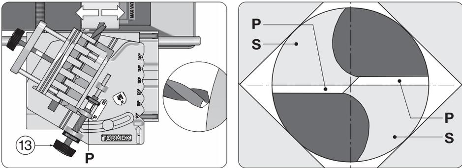
Turn the setting screw (13) lightly towards the grindstone and grind carefully until the 4-facet point is established again.
