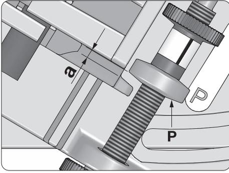
Screw the stop **P** further downwards (**a**) by as much as the tip should be ground. One turn is equal to 0.5 mm (0.02") cutting depth.
