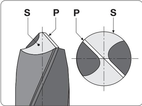
The drill is ground to a 4-facet point. **The Primary facets, P** and the **Secondary facets, S** meet in the centre and form a point.
