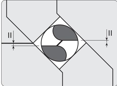
Loosen the wheel and rotate the drill so that the cutting edges are aligned parallel to the horizontal lines on the Drill Holder. Tighten the wheel. The protrusion **L** does not need to remain exact.
