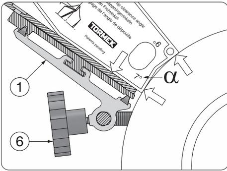
**The clearance angle,  $\alpha$ .** Here 7°. Tilt the Base (1) so that both corners of the Setting Template touch the grindstone. Lock it securely with the wheel (6).
