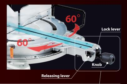
Once Releasing lever is pushed down:
